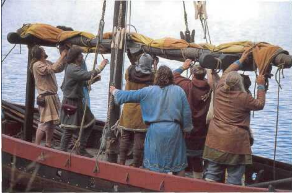
(Left) The Gokstad ship had T-shaped poles forward and aft of the mast on which the yard could be laid when the sail was taken down; here the sail is reefed to the yard for stowage. If the oars had to be used the sail was most probably always taken down - at such times it was not only useless but actually worked against the rowers.
